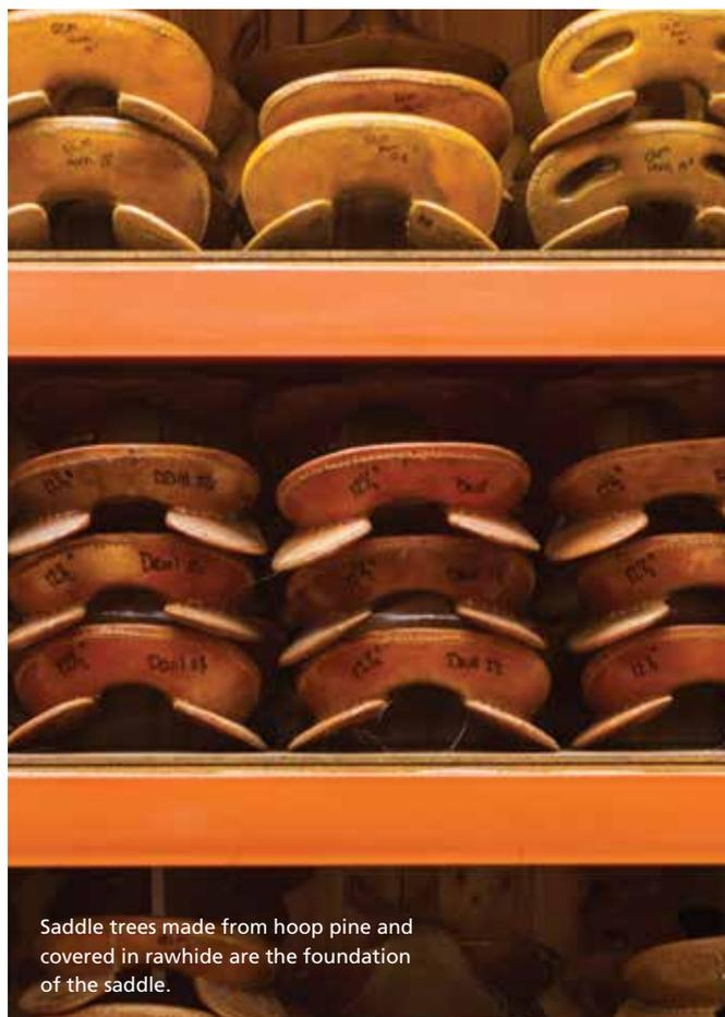
Saddle trees made from hoop pine and covered in rawhide are the foundation of the saddle.
